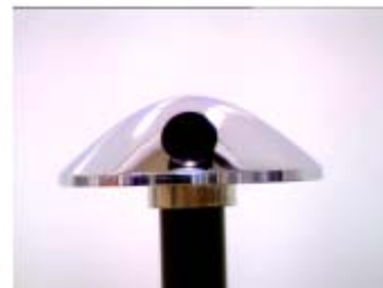
Central Panoramic Camera. Standard perspective camera with hyperbolic mirror II.
