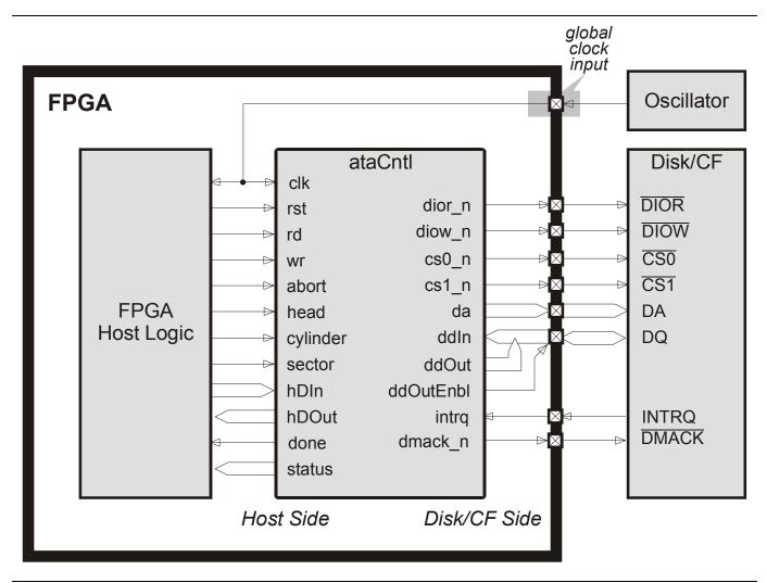
Figure 1: ATA controller connections.
