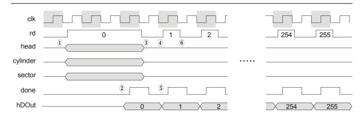
Figure 2: ATA controller read sector waveforms.
